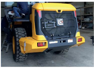
All-around visibility is supported by a rear-view camera acting as an extra eye on the jobsite.
