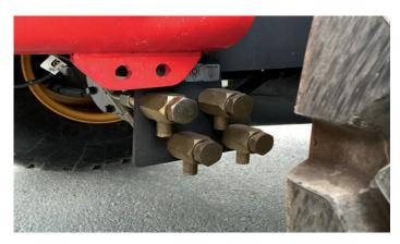
All pressure taps and sight gauges are easily accessible. Fluid drains provide environmentally friendly drainage capability and are grouped together for convenient serviceability.
