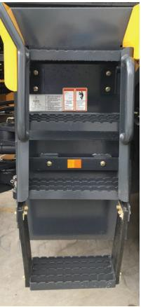
Access to the front of the cab by the operator or service person is a new feature. The same anti-slip bars used on the egress steps are used here for maximum anti-slip protection.
