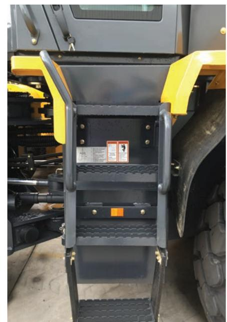
Access to the front of the cab by the operator or service person is a new feature. The same anti-slip bars used on the egress steps are used here for maximum anti-slip protection.
