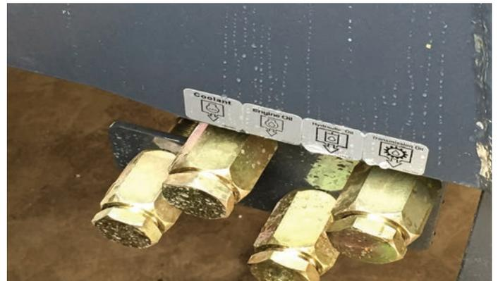
All pressure taps and sight gauges are easily accessible. Fluid drains provide environmentally friendly drainage capability and are grouped together for convenient serviceability.
