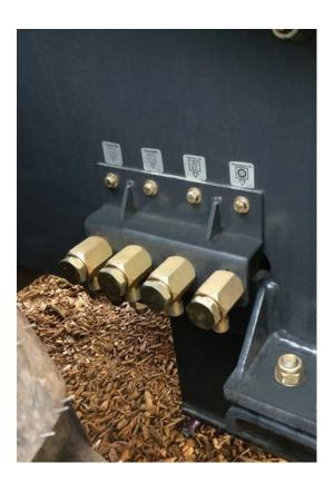
All pressure taps and sight gauges are easily accessible. Fluid drains provide environmentally friendly drainage capability and are grouped together for convenient serviceability.
