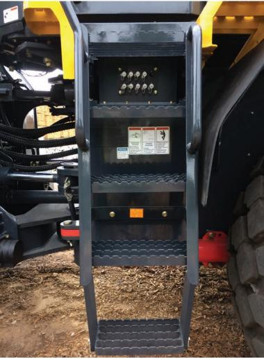
Access to the front of the cab by the operator or service person is a new feature. The same anti-slip bars used on the egress steps are used here for maximum anti-slip protection.
