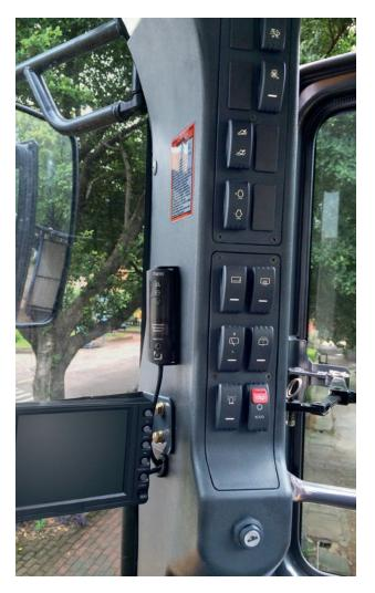
All-around visibility is supported by a rear-view camera acting as an extra eye on the jobsite.
